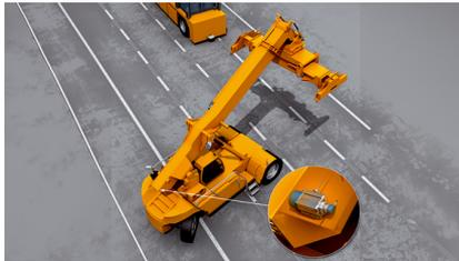
When winding and unwinding, the wire forms not several, but only one row on the measurement drum. This ensures a high measurement accuracy.
