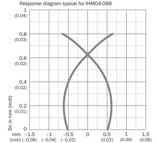
Distance of target edge to center of active face in mm (inch) All dimensions in mm (inch)
