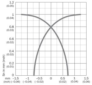
Distance of target edge to center of active face in mm (inch)
