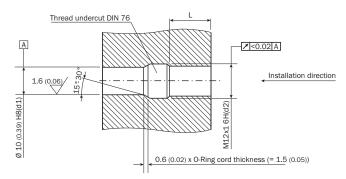
L: recommended installation depth: L  $\geq$  0.8 (0.03) x d2
