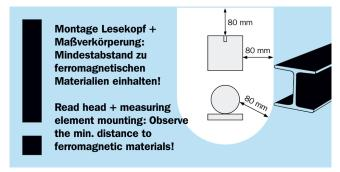
Only use non ferro-magnetic materials for the assembly base of the read head. A separation distance of 80 mm must be observed for ferro-magnetic materials (e.g., iron).
