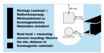
Only use non ferro-magnetic materials for the assembly base of the read head. A separation distance of 80 mm must be observed for ferro-magnetic materials (e.g., iron).
