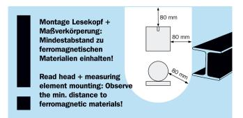
Only use non ferro-magnetic materials for the assembly base of the read head. A separation distance of 80 mm must be observed for ferro-magnetic materials (e.g., iron).
