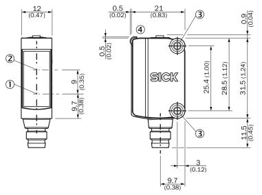
① Center of optical axis, sender
