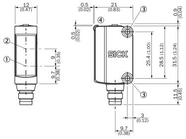
① Center of optical axis, sender
