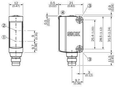
① Center of optical axis, sender
