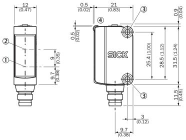
① Center of optical axis, sender
