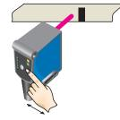
When setting the contrasts to be detected, the first LED (green) flashes in the bar graph. Press Teach-in pushbutton.
