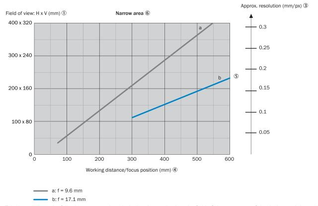
Take into account the following aspects when designing the application: the field of view geometry of the device, and the position of the field of view in the space in front of the device. Possible angles at which the objects can arise in relation to the device. For the planned working distance: resultant field of view length and width as well as the approximate resolution.
