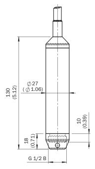
Enhanced variant with FEP cable (immersion depth up to 100 m)
