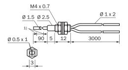
Flexible end tip, do not bend in this area (10 mm), bend radius R10 mm
