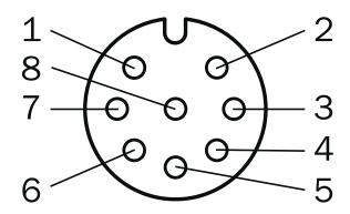
Female connector M12, 8-pin, A-coded
