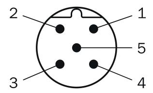
Male connector M12, 5-pin, A-coded
