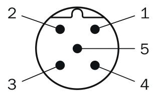
Male connector M12, 5-pin, A-coded
