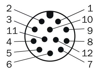
M12, 12-pin male connector, A-coded
