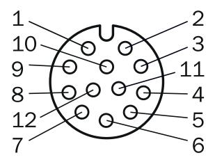
M12, 12-pin female connector, A-coded
