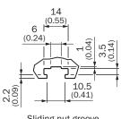
Sliding nut groove for side mounting
