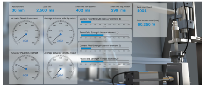
Traversing speed, cylinder travel, dwell time in the end positions and magnetic field strength are only some examples of diagnostic data the MPS-G generates
