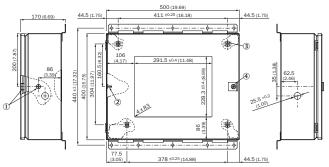
① Earth connection (acc. to VDE-0100, Part 410), specification: See manufacturer's drawing
