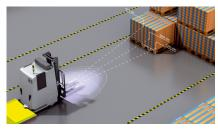
The MRS1000 allows for correct positioning of the transport fork of an automated guided vehicle during the approach and reception of the pallet without stopping the AGV.
