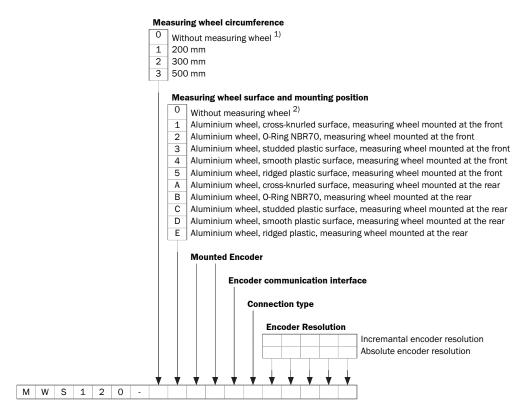
$^{(1)}$  Not in combination "Measuring wheel surface and mounting position" 0 and "Mounted encoder" 00.
