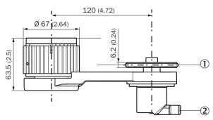
① The measuring wheel circumference and surface depend on the installed measuring wheel.
