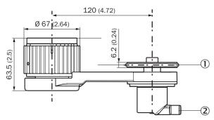
① The measuring wheel circumference and surface depend on the installed measuring wheel.
