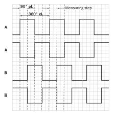
The measuring step corresponds to 90° electrical. The measuring step  $[\mu m/pulse]$  specified under Performance can only be achieved if the output signals of the sensor are evaluated differentially.
