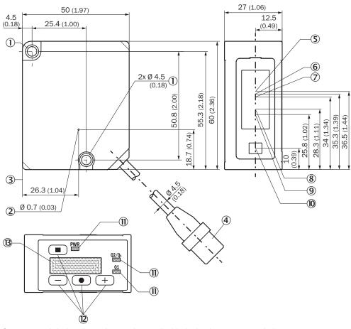
Structure and device dimensions, unit: mm (inch), decimal separator: period
