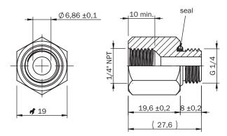
Bottom: 1/4" NPT female thread, pre-installed NPT adapter in G 1/4 female thread; rear: G 1/4 female thread
