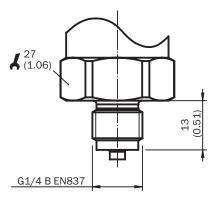
Housing with L-connector (DIN 175301-803 A), IP65
