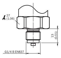
Housing with L-connector (DIN 175301-803 A), IP65
