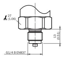
Housing with L-connector (DIN 175301-803 A), IP65
