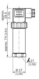
Process connection with flush-mounted membrane, G  $\frac{1}{2}$  B with/without cooling element, 0 ... 2.5 up to 0 ... 600 bar, max. overpressure safety 600 bar
