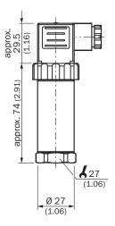
Process connection with flush-mounted membrane, G 1 B with/without cooling element, 0 ... 0.1 up to 0 ... 1.6 bar
