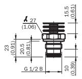
Housing with L-connector (DIN EN 175301-803 A)
