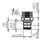
Housing with L-connector (DIN EN 175301-803 A)
