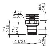
Housing with L-connector (DIN EN 175301-803 A)
