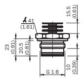
Housing with L-connector (DIN EN 175301-803 A)
