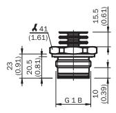
Housing with L-connector (DIN EN 175301-803 A)
