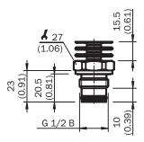
Housing with L-connector (DIN EN 175301-803 A)
