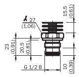
Housing with L-connector (DIN EN 175301-803 A)
