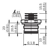
Housing with circular plug-in connector M12 x 1
