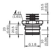
Housing with L-connector (DIN EN 175301-803 A)
