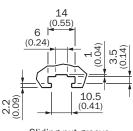
Sliding nut groove for side mounting
