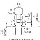
Sliding nut groove for side mounting
