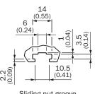
Sliding nut groove for side mounting
