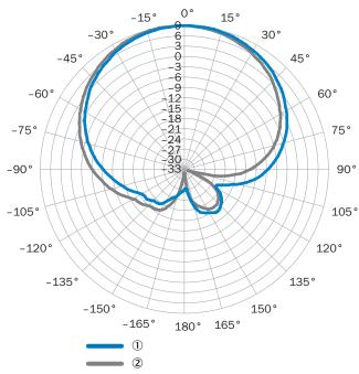
Measured antenna gain in dBic at 868.5 MHz, RHCP (right-hand circularly polarized)
