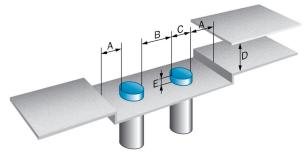
Distances required to prevent mutual interference with parallel mounting of several devices as well as from the environment. RFH505/510 (in metal)
