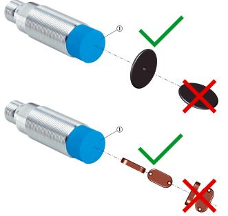
Optimal alignment of the transponders for a reliable read and write process O process the transponder of transponder of the transponder of trans
