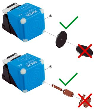
Optimal alignment of the transponders for a reliable read and write process 1 Cap with integrated antenna
