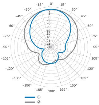
Measured antenna gain in dBic at 866.5 MHz, RHCP (right-hand circularly polarized)
