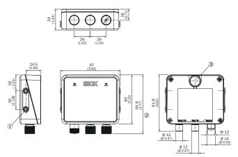
Structure and device dimensions, unit: mm (inch), decimal separator: period
